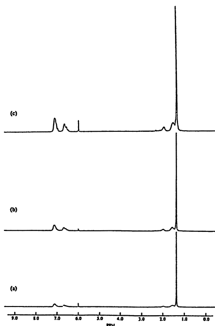
Figure 10. The 1 H NMR spectra of PE-g-PS copolymers, containing (a) 25.6 (b) 38.1 and (c) 43.8 mole % of polystyrene.
